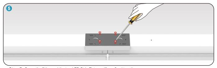
**Step 5** Screw the fitting and the two LED Strip Fixtures 4ft are fixed together.
