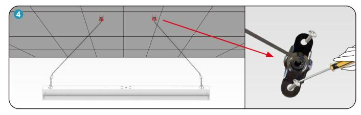
**Step 4** Screw the top of the lanyard to the top of the office to complete the installation.
