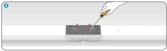
**Step 5** Screw the fitting and the two LED Strip Fixtures 4ft are fixed together.
