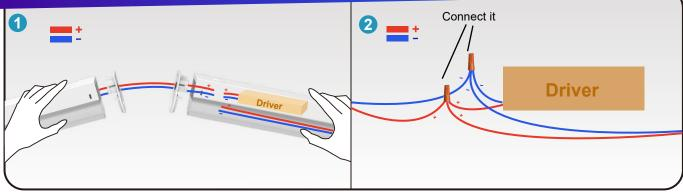
**Step 1** First open the lid at both ends of the LED, then pass the positive and negative wires through the two lids.
