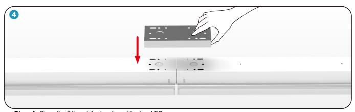
**Step 4** Place the fitting at the junction of the two LEDs.
