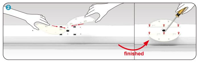
**Step 2** Insert the two mounting plug-ins diagonally into the lamp body, Then screw on the screws.
