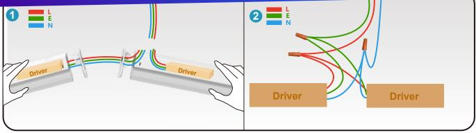
**Step 1** First open the lid at both ends of the LED, Then the live wire, neutral wire and ground wire pass through the two covers.
